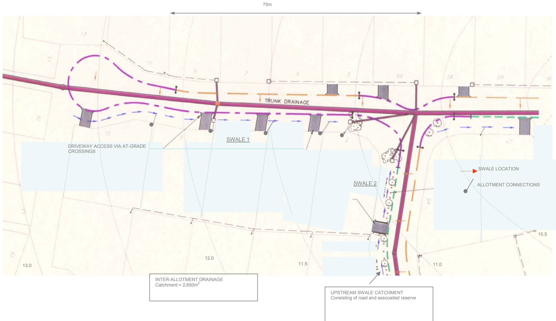
Figure 2-16: Typical Layout for Swale Worked Example
