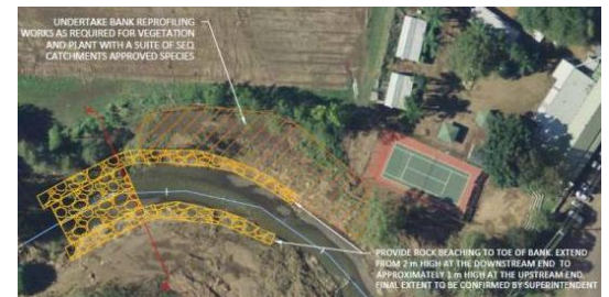
Bank battering involves setting back the bank to reduce the steepness. Associated infrastructure may need to be relocated. A mix of vegetation including groundcover, shrubs and trees need to feature in the final solution.
